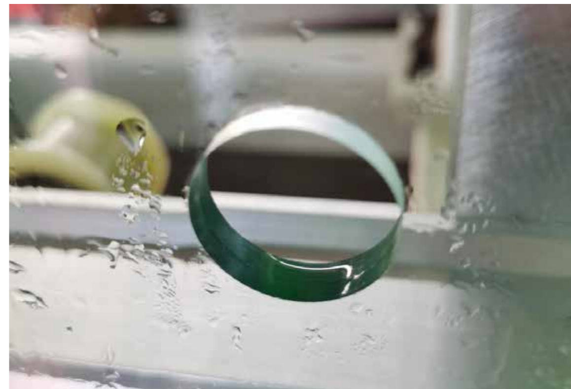
Samples processed by vertical glass drilling and milling machine:
